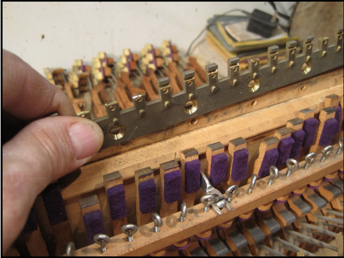
Brass rail with multiple problems being removed for duplication.
